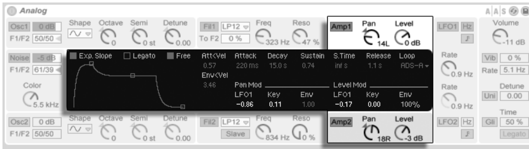
Display and Shell Parameters for the two Amplifiers.
